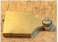
A steel washer bolted to the blank makes a good guide for cutting & smoothing the top of the LC
