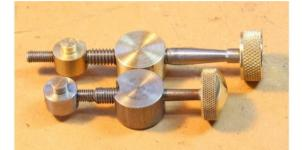
Both adjusters fully extended. The total range of travel in the modified version is about 7mm vs 13mm for the original
