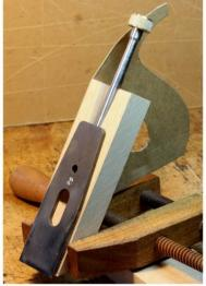
Checking that the blade has sufficient travel & the shaft matches proposed handle shape
