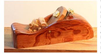
than wedges or perhaps a good marketing point. But screwed lever-caps & screw adjusters are certainly complementary; loosening & tightening wedges in order to adjust blade depth would become very tedious and essentially negate any convenience the adjuster offered (which to be honest, is not all that much once you get used to hammer setting). This is recognised by Veritas who offer a sort of "wedge lever" with their small plane kits – the 'wedge' is
