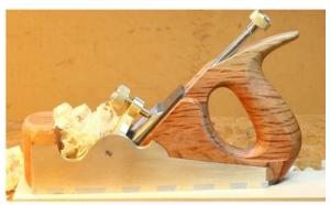
With the modified adjuster the plane is quite easy to set for 0.025mm shavings compared with a Veritas adjuster.
