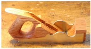
Large channel in blade bed needed to accommodate the longer adjuster shaft
