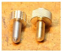
Thumbscrew made by hand-knurling compared with one made using a knurling tool
