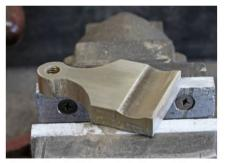
Cove refined with a coarse half-round file and sandpaper wrapped round a suitably-sized dowel
