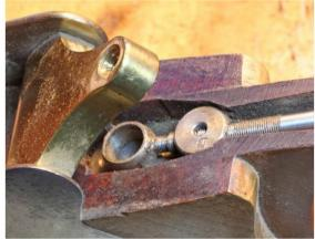
Norris adjuster: note cup or 'banjo' which receives the cap-iron screw. These adjusters require a large excavation in the blade bed.
