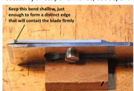
pressure is applied by the lever-cap, you *could* promote a 'springy' blade prone to chatter, so I think it's always safer to have the blade as flat & straight as possible. The old wooden planes & infills had very thick, single bend cap-irons, but they also had very thick blades (of the order of 6mm) which resisted flexing.
