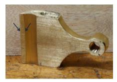
To get a clean, straight, mating surface at the toe, I first file a back-bevel on the underside of the leading edge to obtain a distinct lip (arrowed at left) with enough relief that only a narrow strip 1-2 mm wide actually contacts the blade or capiron. File carefully to avoid forming a curve, which is all too easy to do. The lip can be further flattened by carefully stroking it over a sheet of tightly-stretched sandpaper until it is perfectly straight.
