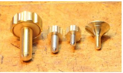
Home-made thumbscrews. L to R: large TS made from a brass hose fitting ; two made from stainless steel bolts and heads of hand-knurled brass rod; TS made from brass cupboard knob and M6 brass bolt.
