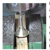
bolt of suitable size. In the case illustrated at left & right, I used a 20mm knob and a 6mm bolt to make a thumbscrew for a small (110mm) plane.
