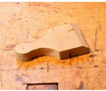
the mock-up (taps for metal work quite well in wood across the grain), & by adding the thumbscrew, get a clear idea of how the LC fits.
