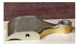
Lever cap with cove under toe and shaping of neck
