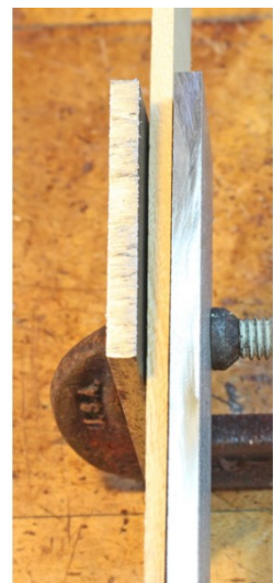
Hacksaw cut (left) compared with disc cut
