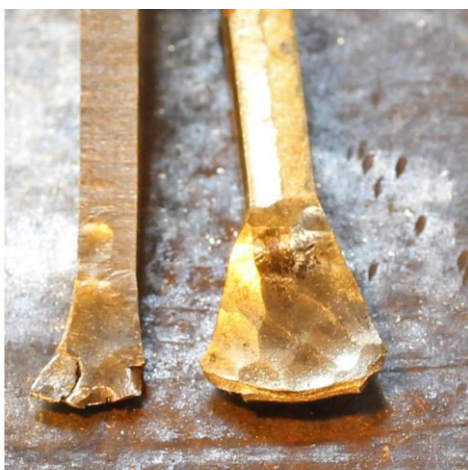
C385 brass (left) compared with H62. The more ductile H62 has tolerated heavy hammering & spreading without flaking or splitting.
