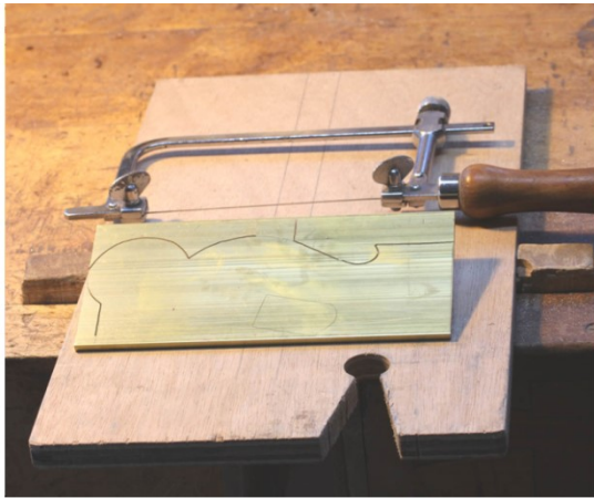
Birds-mouth cutting board. The various cuts needed to remove the waste with the shallow saw are highlighted
