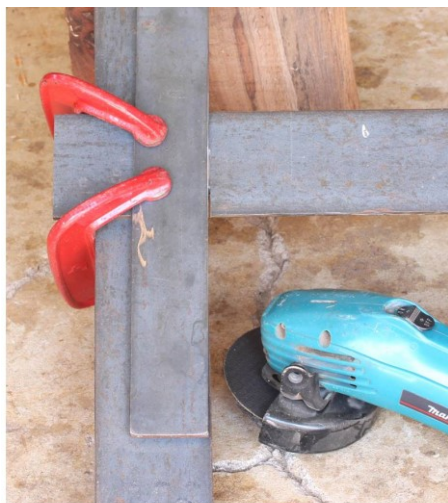
Cutting steel with a 1mm cutoff wheel against a guide
