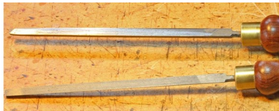
A 6" EST file converted to a pseudo-barette by grinding two safe faces. This is a handy size for most small to medium planes.
