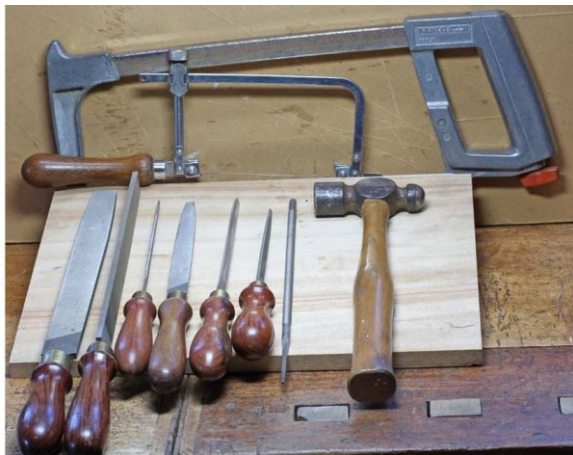
Basic set of tools for making metal-bodied planes
