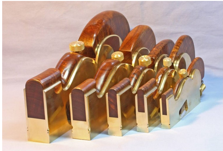
Shoulder planes made by the lamination technique, using each of the readily-available blade sizes, (L to R): 32mm, 25mm, 19mm, 16mm and 13mm
