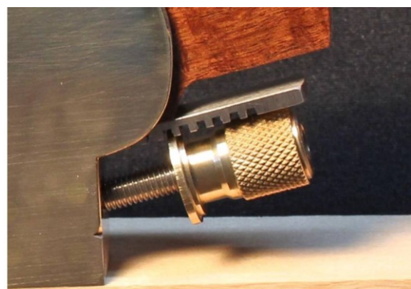
Adjuster fitted to a Mujingfang blade with multiple grooves on tang.
