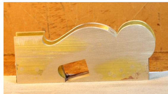
Rivet heads filed flush with sides
