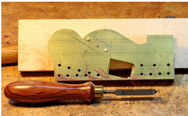
Holes for rivets drilled & countersunk using the home-made tool in foreground
