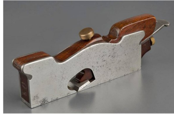
Norris A7 shoulder plane with wedge retained by a thumbscrew
