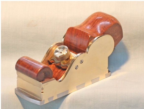
Version 1, with fixed bridge and thumbscrew but no screw adjuster. Blackwood infill
