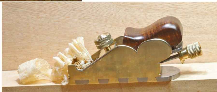
With adjuster and fixed bridge/thumbscrew
