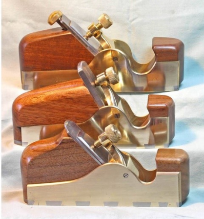
3 small planes made from the same side pattern. Variations include blade angles, curved sides and an adjuster.
