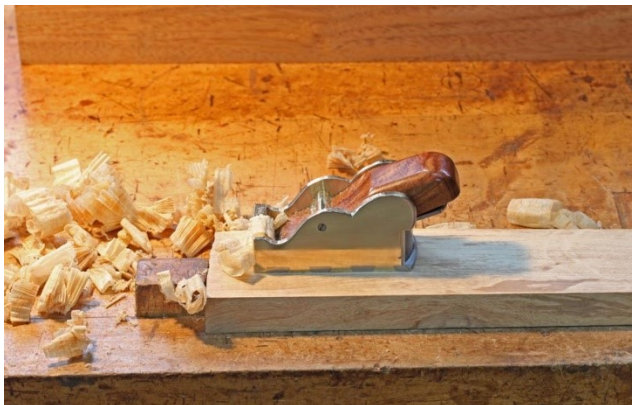
Adjusterless version with swivelling bridge and simple wedge
